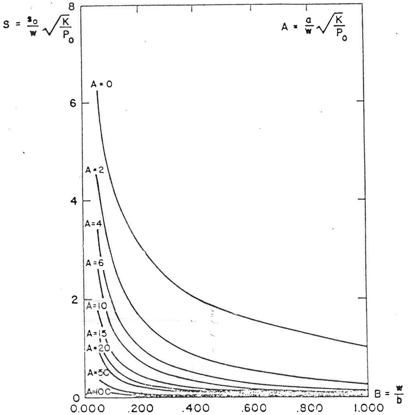
Figure 6. Subsurface drainage design graph.
