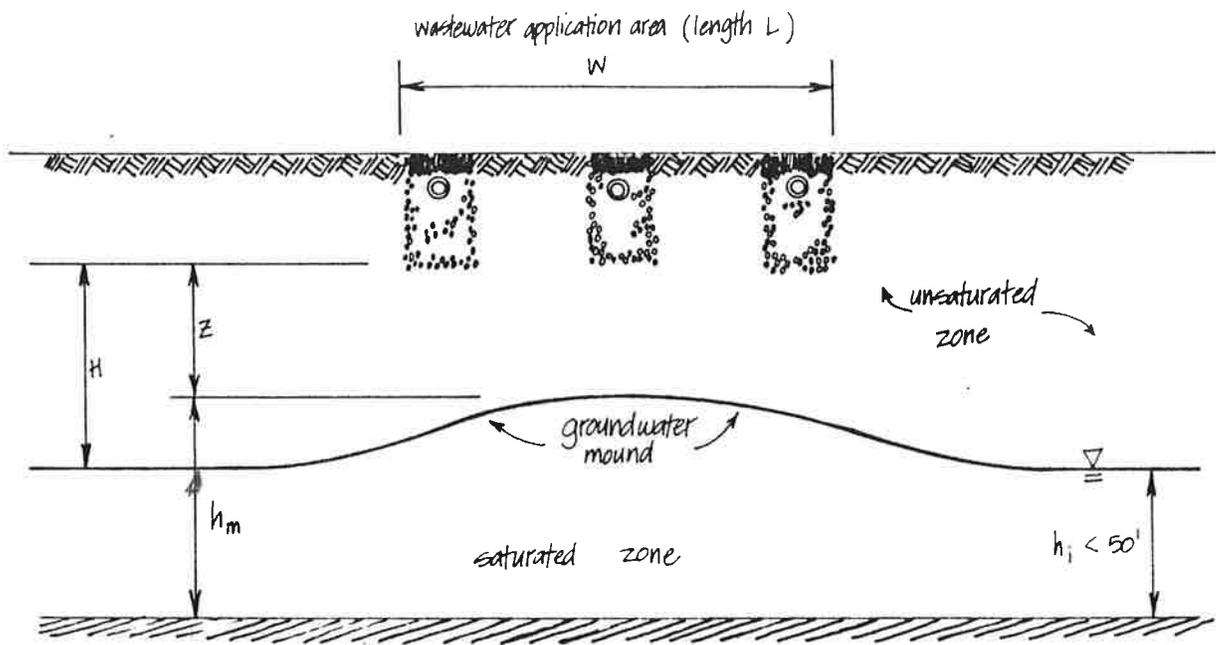
Fig. 4. Groundwater Mounding for Case 2 - Relatively Thin Groundwater Zone
