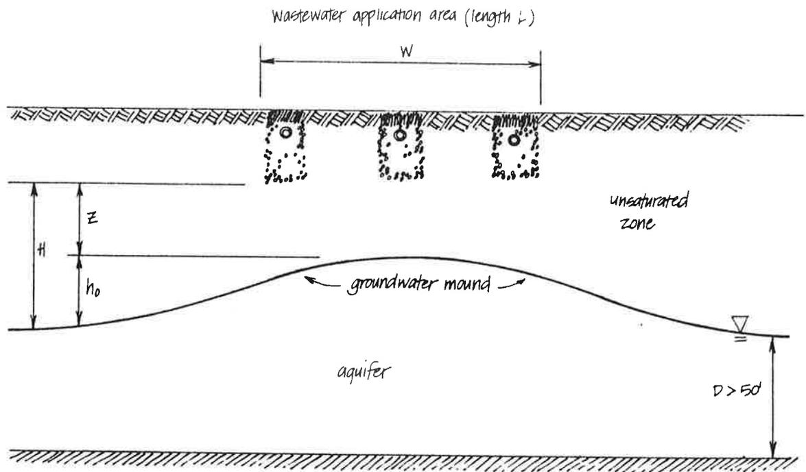
Fig. 2. Groundwater Mounding for Case 1 -
