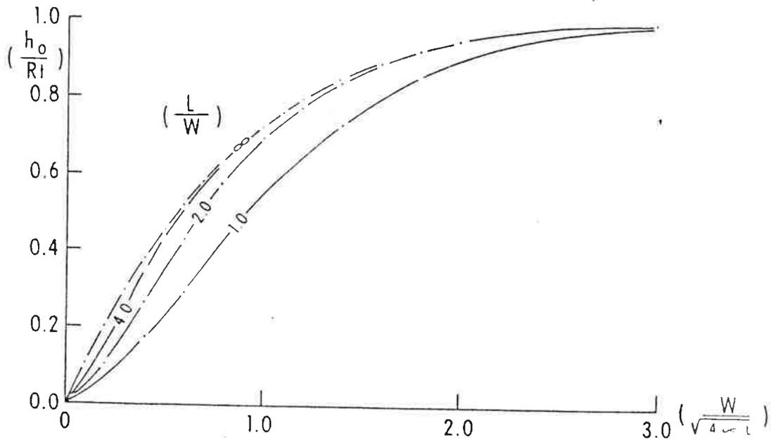
Fig. 3. Dimensionless Plot of the Rise at the Center
