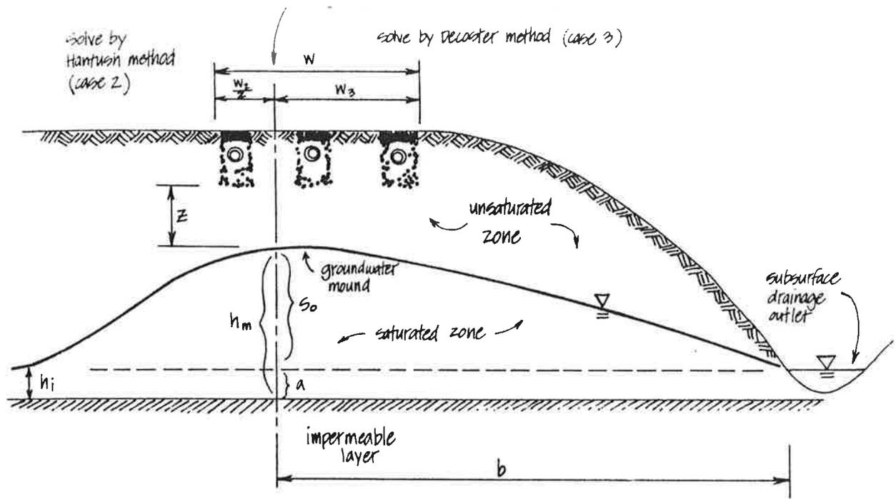
Fig. 7. Combined Application of Case 2 and Case 3 Methodologies
